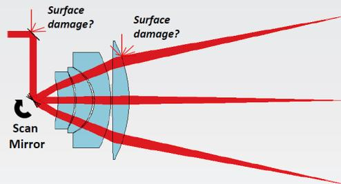
Fig. 1: Illustration of an optical system using a laser light source at levels which may damage the coating on the surface of a lens or mirror within the beam path.
