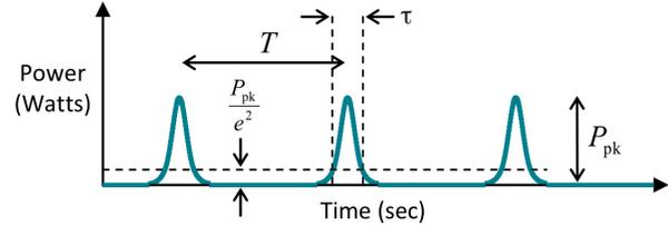
Fig. 4: A pulse train with Gaussian temporal profiles.
