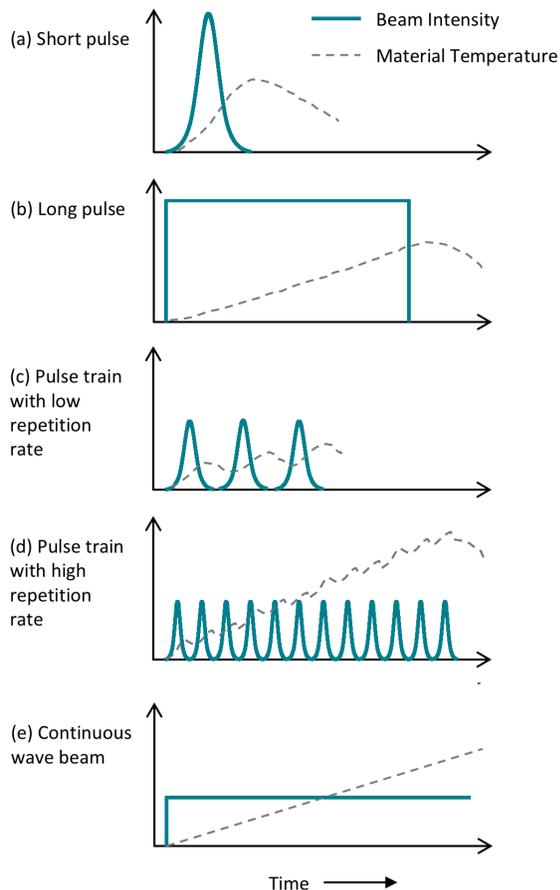
Fig. 2: Illustration of the response of a material's temperature due to absorption of laser beam intensity.
