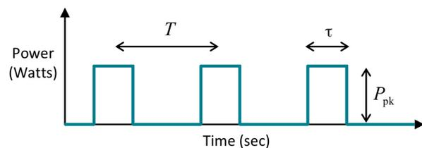
Fig. 3: A pulse train with rectangular temporal profiles.
