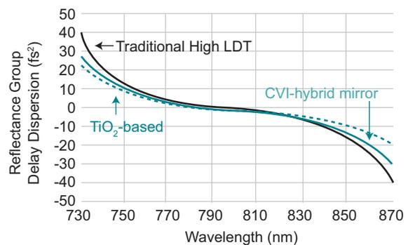
Fig. 6: A comparison of Reflectance Group Delay Dispersion vs. Wavelength of  $\text{TiO}_2$ -based, traditional high LDT, and the new CVI-hybrid mirror.
