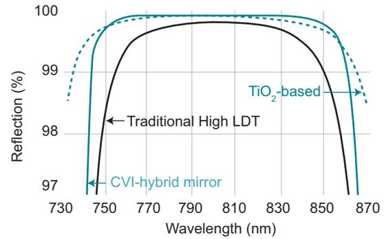
Fig. 5: A comparison of Reflectivity vs. Wavelength of  $\text{TiO}_2$ -based traditional high laser damage threshold (LDT), and the new CVI-hybrid mirror.
